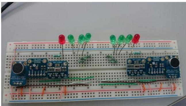
Fig. 2. Protoboard with light, noise, temperature and pressure sensors.
