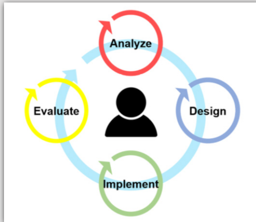
Fig. 3: The user-centered design model. An iterative design process in which designers focus on the users and their needs in each phase of the design process.
