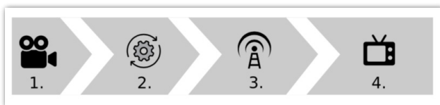
Fig. 4. TV broadcasting pipeline: 1. Camera acquisition and digitalization; 2. Media adaptation and encoding; 3. Air/Sat/Cable distribution; 4. Client reproduction. The whole the process happens in push, from content producers towards end users.
