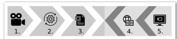
Fig. 3. HTTP Adaptive Streaming video pipeline: 1. Camera acquisition and digitalization; 2. Segmenting and encoding; 3. Video files and playlist assembly; 4. CDN distribution; 5. Client reproduction. The first three steps are executed in a push-oriented video-production process, while the last two are pull-based, initiated by clients.
