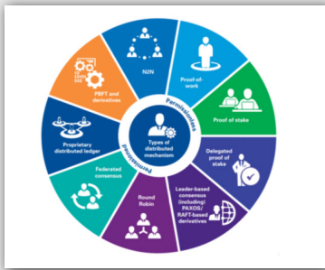
Fig. 4. Taxonomy of different approaches known in the literature to reach consensus in a distributed system. (source: "Consensus: Immutable agreement for the Internet of value" [9])
